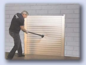
In impact testing, Qompact withstood 82 punches, 5 kicks, and 80 hits with a sledge hammer. The foam-filled shutter was destroyed in seconds.
