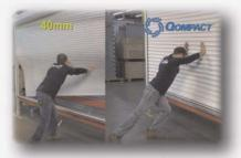
Qompact's end retention prohibits the curtain from being pushed out of the rails. Without end retention, the 40mm foamfilled curtain was easily compromised.
