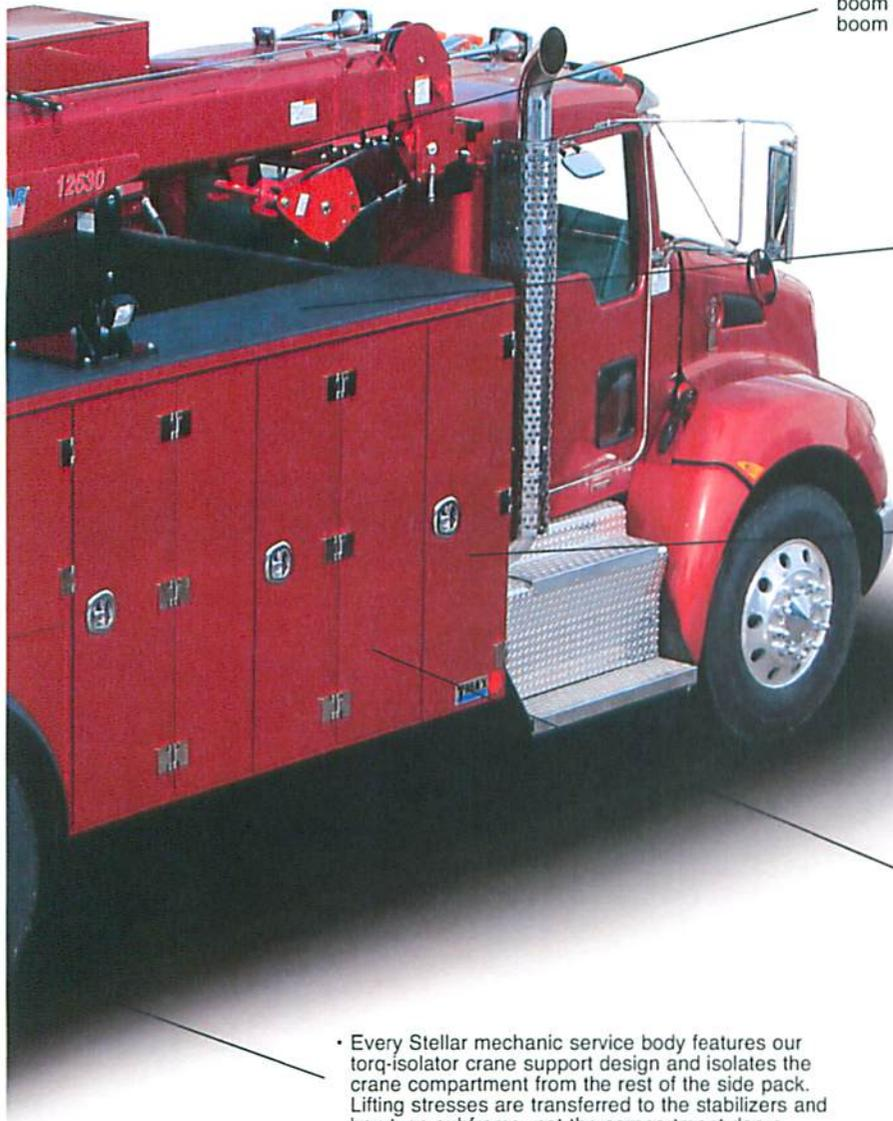
• The Stellar TMAX mechanic service body uses a roller type boom support. The roller boom support helps to center the crane boom when stowing.
