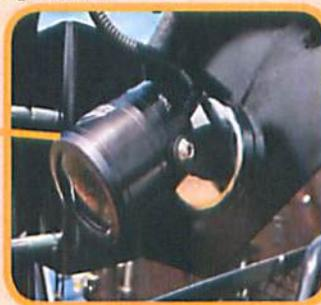
Optional camera located on the right side of the TrucKat allows the operator to view the cutting head in operation while facing forward and steering vehicle.
