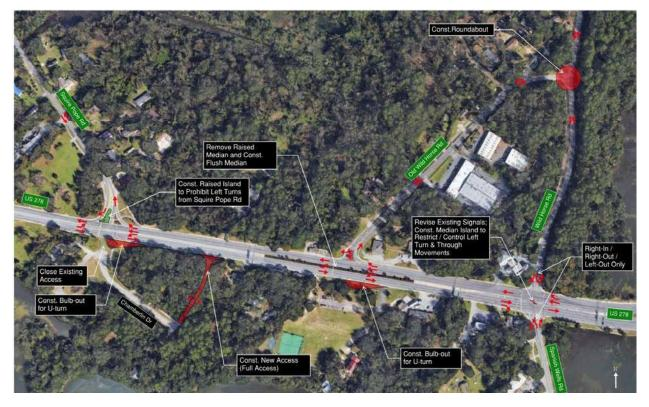
Figure 5. Two-Phase Signal Alternative
